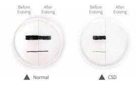
It can be seen that the CSD lens is easier to erase the writings and nearly can be without any small tiny trace. The excellent oleophobicity makes the grease dirt not easy to adhere on the lens, effectively reducing the trouble of stains, makes you not to worry about the oil, fingerprints and dust in the air which can make the lens blur. The easiness for cleaning makes the vision clearer and brings a different sensory experience for you.
